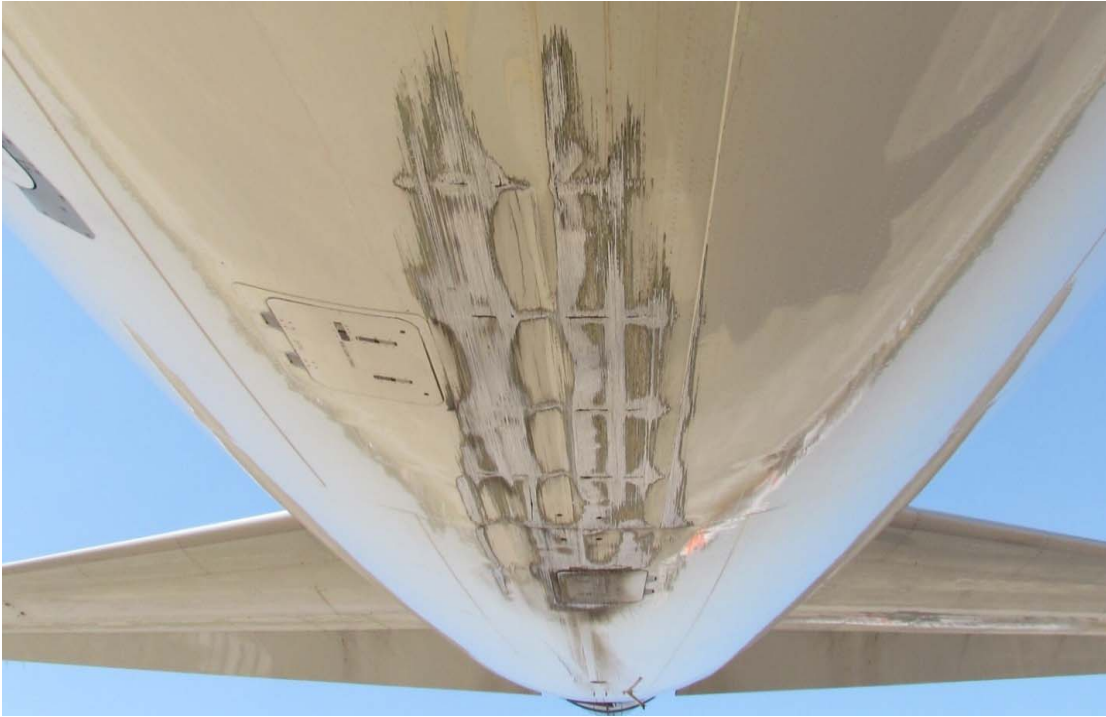
Figure (4) Scrape marks on aircraft tail section
